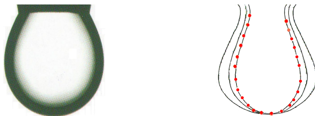
Figure 1. Drop (a) and its coordinate (b - points); curves calculated for different values of surface tension.
