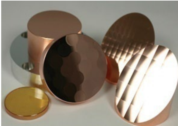
Figure 12. Optical elements high power CO 2 laser covered by diamond films [75].
